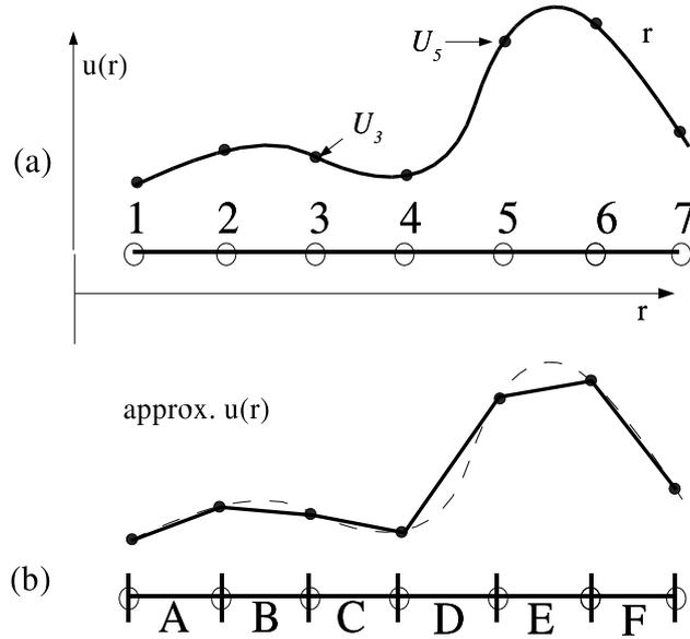
Figure 6: 1D example of interpolation with linear elements. In (a), the exact function is shown, whereas (b) shows the interpolated function given the exact values  $U_i$  at each node.
