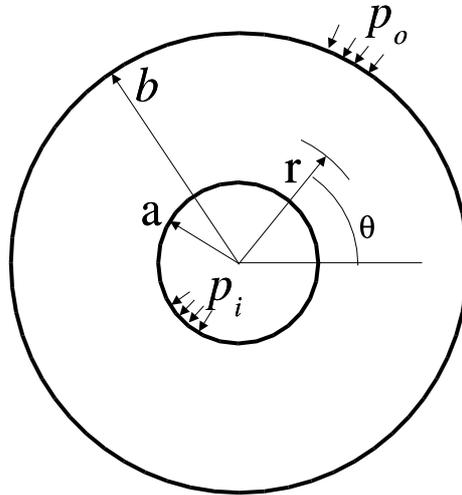
Figure 7: Pressurized cylinder.
