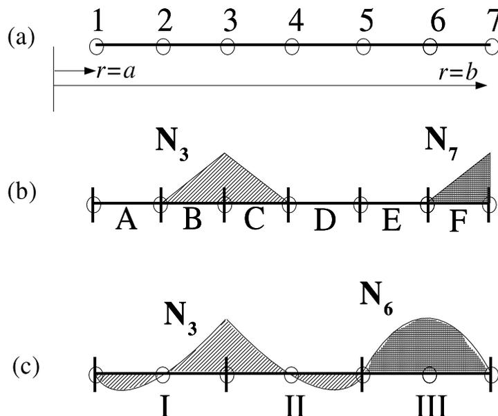
Figure 4: Shape functions for a one-dimensional domain. (a) Discretized domain. (b) Linear Elements A-F. (c) Quadratic Elements I-III.
