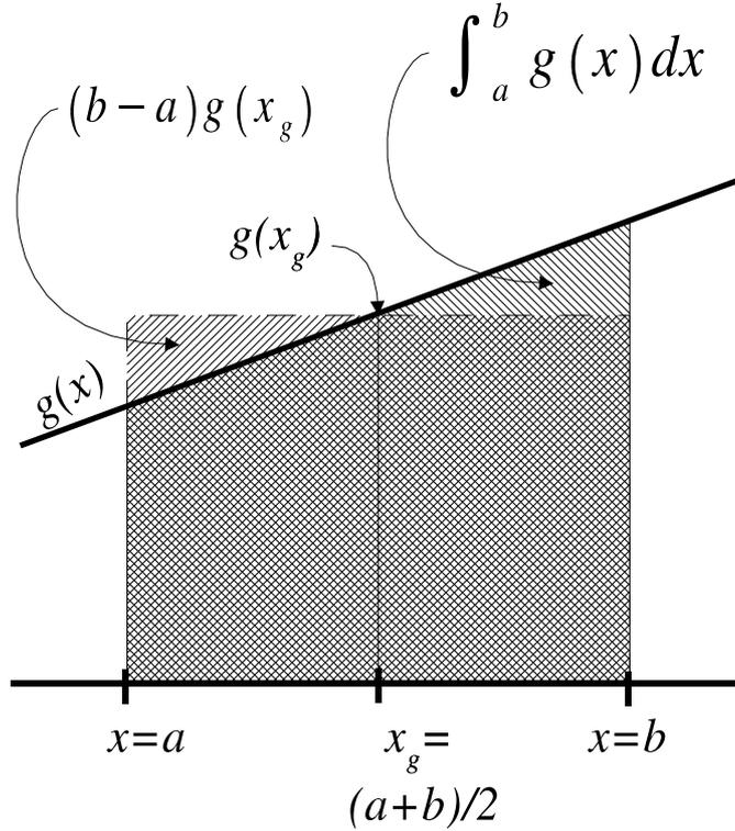
Figure 8: Gaussian quadrature of a linear function.
