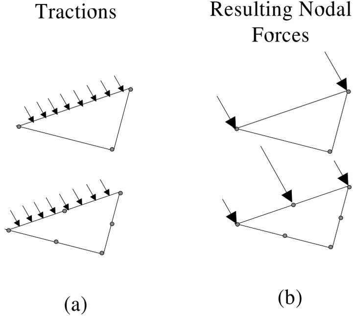
Figure 9: Schematic of the result of integrating the applied tractions. (a) Applied tractions. (b) Equivalent forces lumped onto nodes.
