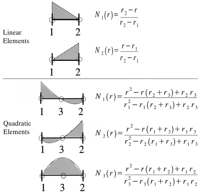
Figure 5: Linear and Quadratic Elemental Shape functions for a one-dimensional domain.
