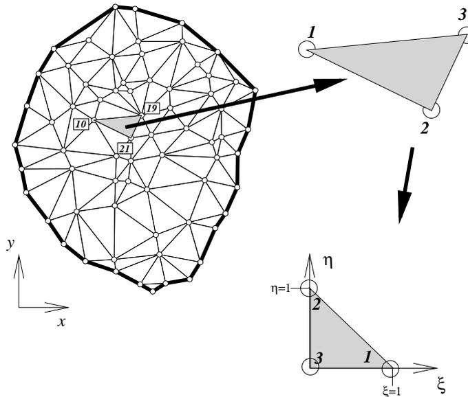
Figure 11: Elements of arbitrary size and shape are first referred to a local node numbering scheme, and then mapped to a parent element for efficient implementation.
