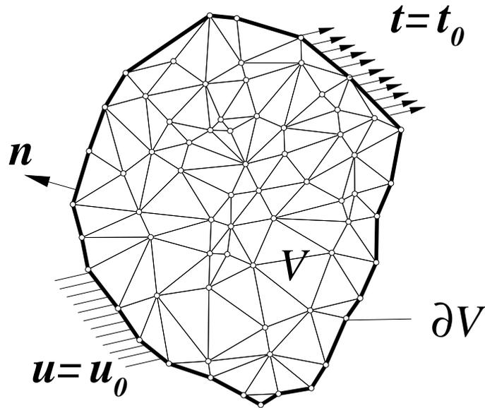
Figure 3: Elements connecting the nodes to form a finite element mesh.
