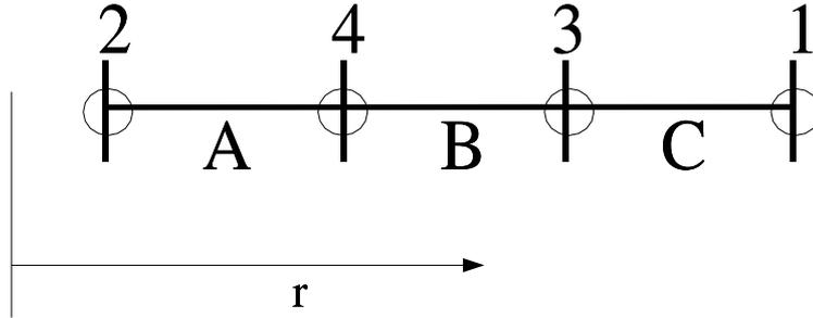
Figure 10: Simple one-dimensional mesh with three linear elements and four randomly numbered nodes.
