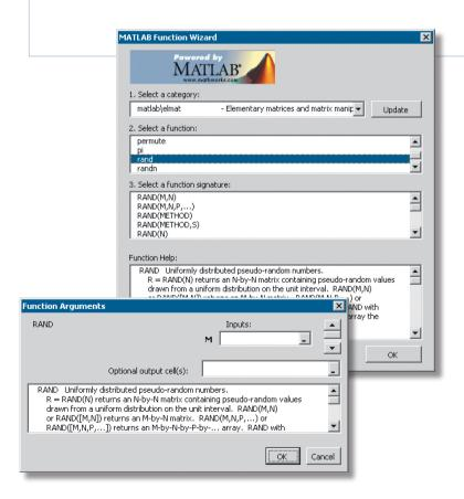
The MATLAB® Function Wizard for Spreadsheet Link $^{\text{\tiny TM}}$  EX. You can browse MATLAB® directories and functions from Excel $^{\text{\tiny SM}}$  and run selected functions from an Excel spreadsheet.
