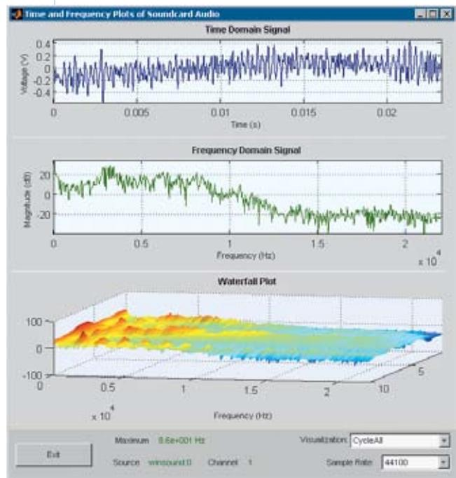
Spectrum analysis application, deployed and running outside MATLAB on Windows. The application, developed in MATLAB, directly acquires signals from a data acquisition board and performs data analysis and plotting.
