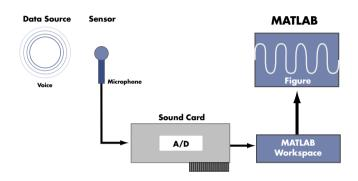
Setup for a data acquisition and analysis session. The Data Acquisition Toolbox enables MATLAB to interface with the data acquisition boards, such as sound cards.
